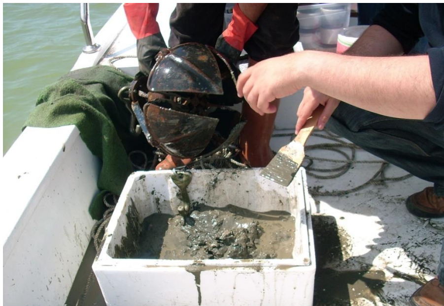
Picture 6. Sediment grab and sediment sample
