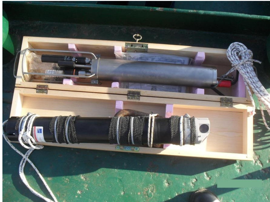
Picture 2. CTD and current meter used in the sampling provided by the Project coordinator
